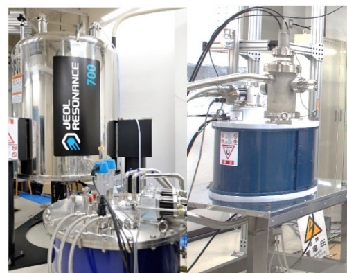
Figure 2 Ultra-highly sensitive DNP-NMR spectrometer. A superconducting magnet (left) and a terahertz-wave light source, a gyrotron (right), are used to observe NMR at cryogenic temperatures.
